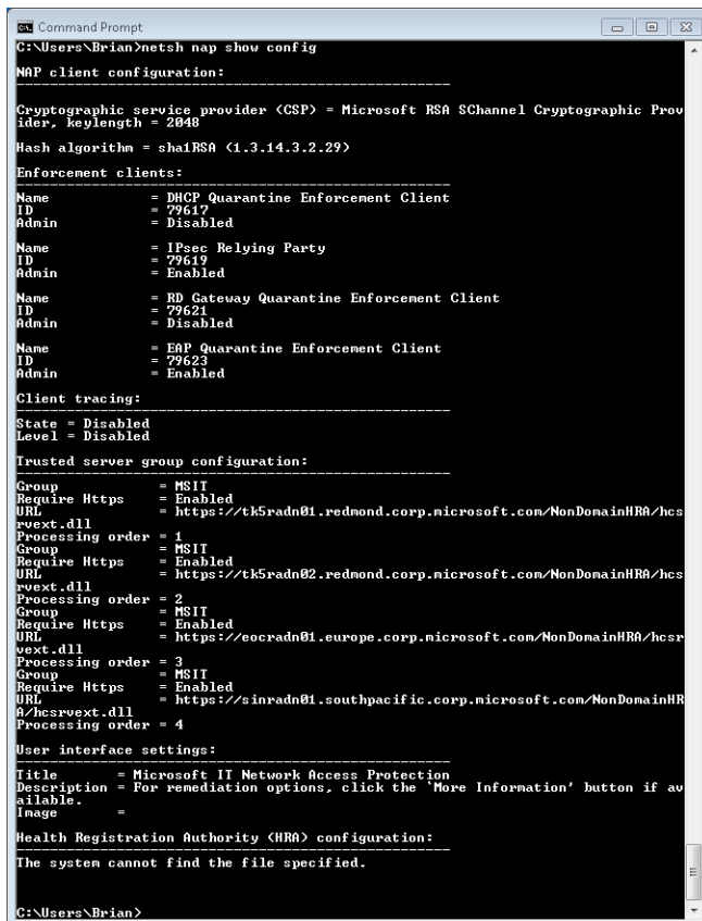
FIGURE 7-53 Configuring NAP using the network shell
